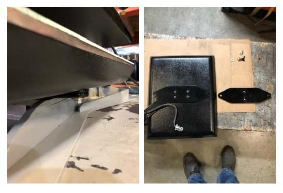
ATTACH the bottom heat assembly to the Black Mounting Plate using (2) 5/16-18 screws. The mounting holes are outside the machine base-frame area for easy tightning.
